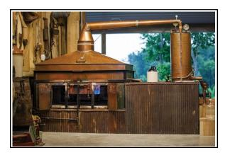
This style of still also had less parts than others making it quicker and easier to set up and take down.
